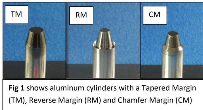
**Fig 1** shows aluminum cylinders with a Tapered Margin (TM), Reverse Margin (RM) and Chamfer Margin (CM)
