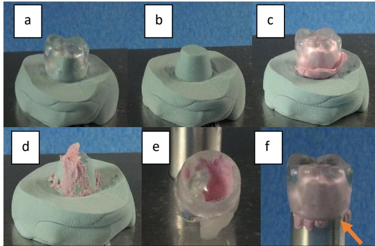
**Fig 6** Clear crown (a) is used to make the replica (b) to push excess cement (DAP) out of the crown (c). Remaining cement on replica after removal of crown. (d) Cement remaining on inside of crown. (e) Crown seated onto Tapered Rod. (f) Arrow shows entrance to cement void on margin. Note uneven ejection of cement.
