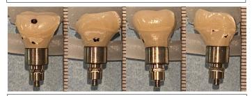
**Figure 6:** Photographs of CMS crowns positioned adjacent to ruler with mm markings to measure cement travel beyond their buccal (B), mesial (M), lingual (L) and distal (D) margins. Black markings highlight extent of cement travel.
