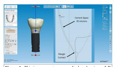
**Figure 1:** This is a computer-screen display showing a 3-D view of a CMS crown, abutment, and implant-analogue complex with a cross-sectional view on the right. The cement space was set to 45 microns and the crown was designed to sit directly onto the abutment margin. The emergence profile of the crown is convex and wider than the abutment.
