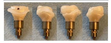
**Figure 7:** RMS crowns are cemented onto their abutments and attached to their implant analogues. Excess cement is above the abutment margins, unlike CMS.
