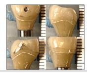
**Figure 8:** Excess cement was removed to display the CMS abutment to crown interface. The vertical height of the opening was measured on the computer display in reference to the adjacent mm ruler grid.
