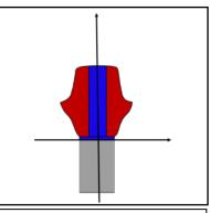
**Figure 2:** The axes of the abutment (red & blue) and implant connectors (grey) are the same and determined by the geometry of the connecting parts. There is nothing to prevent the optimal seating of the abutment. The Government testing is done in a laboratory rather than in the mouth.
