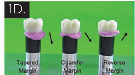
Figure 1 C—Shows 3 aluminum rods with different margin designs. D—Shows the rods with zirconia crowns cemented into place. The arrows indicate the direction of the margins and the cement flow. Note, the Tapered and Chamfer Margin designs direct the cement downwards while the Reverse Margin directs the cement upwards.
