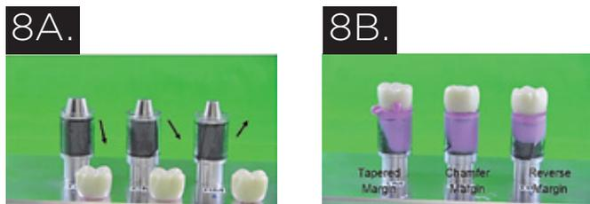
**Figure 8—A** Shows 3 aluminum rods with 3 different margin designs that terminate 1 mm below the top of the clear Tygon tubes (gingiva). The black electrical tape was placed 1 mm below the margin and is 0.125 mm thick. It fills the space between the tube and the rod. The black arrows indicate the direction of the margins. **B—**Depicts the zirconia crowns cemented into place. Note the huge amount of sub-margin cement, regardless of margin design.
